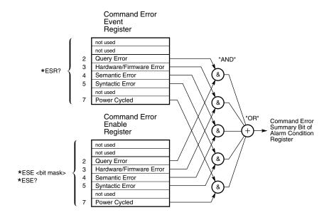
Figure 5-4. Command Error Event and Enable Registers
