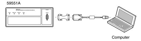
Figure 2-4. Connecting the 59551A to Laptop Computer
