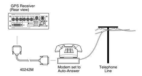
Figure 2-3. Connecting the GPS Receiver to a Modem
