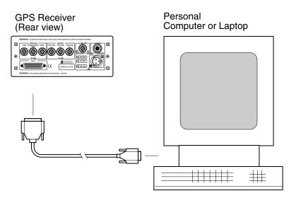
Figure 3-1. Connecting the GPS Receiver to a Computer
