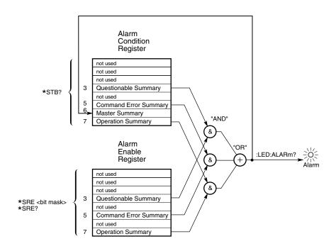
Figure 5-2. Alarm Condition and Enable Registers
