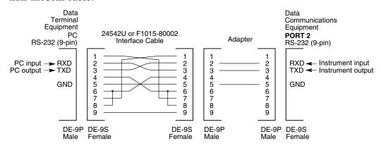
Figure 2-5. DB-9 to DB-9 Serial Connection
