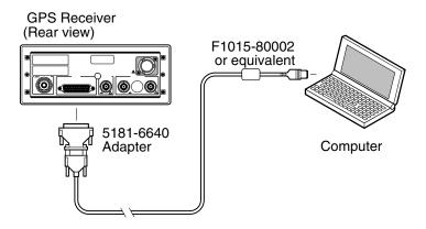
Figure 2-2. Connecting the GPS Receiver to a Computer
